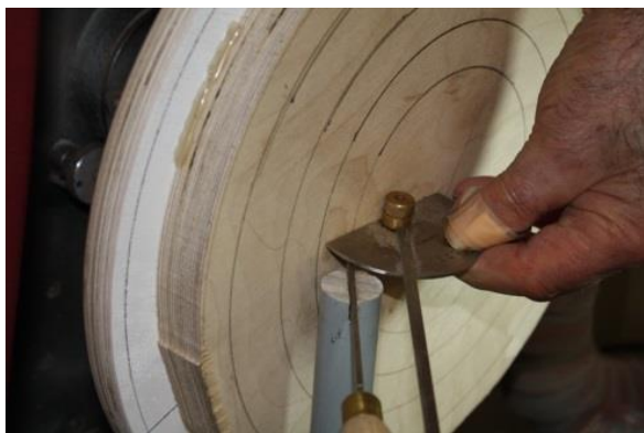
Figure3: Setting the parting tool angle.
